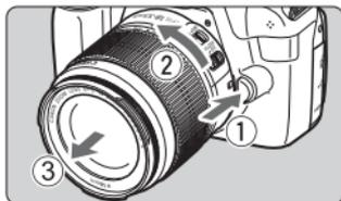
**While pressing the lens release button, turn the lens as shown by the arrows.**
