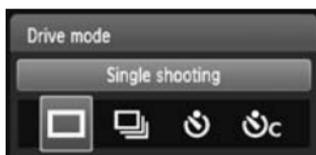
When you press <SET>, the drive mode or flash firing setting screens will appear. Set as desired, then press <SET> to finalize the setting and return to the Quick Control screen.
