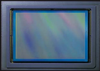
Canon Full-Frame CMOS Sensor — The EOS-1Ds Mark III and EOS 5D come with a newly developed, full-frame CMOS sensor, so it is possible to shoot with any EF lens without a conversion factor.
