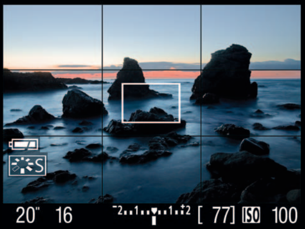
EOS 40D’s Live View function lets you compose and shoot directly from the camera’s 3.0-inch LCD screen.
